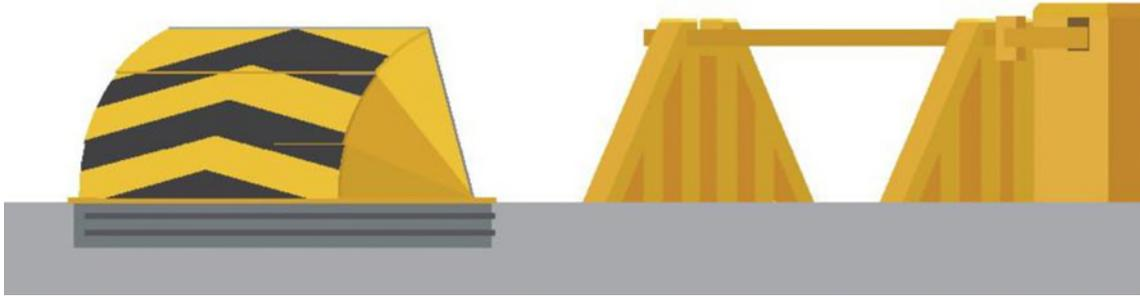
An active VSB can be manually operated by a person or powered (e.g. hydraulic power source). A VSB should be selected not only on the basis of performance or operational requirements, but also cost. Careful consideration should be made by the consultant and purchaser as to the full cost of a VSB, especially post- installation costs and long-term requirements such as:
